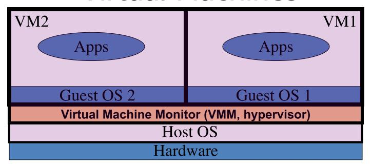
single HW platform with isolated components
