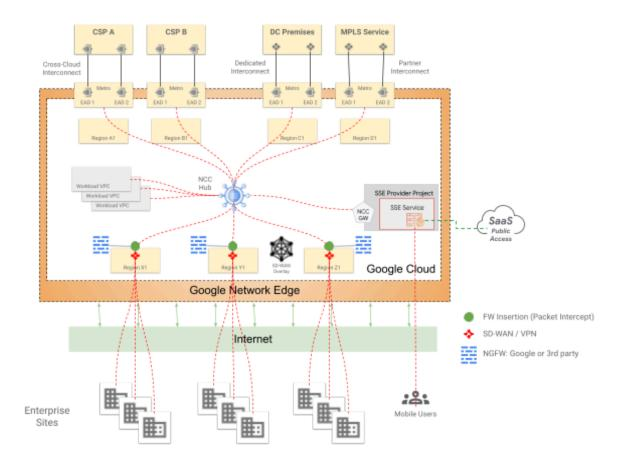
The packet interception model is also instrumental in enabling efficient internet egress security with network address translation (NAT) and proxy services for URL filtering using Secure Web Proxy (SWP). SWP can be deployed as a service leveraging the Private Service Connect (PSC) producer-consumer
