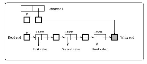
Figure 1: A channel with unbounded buffering
